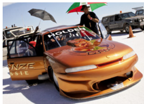
Rod Hadfield's car The Bronze Aussie is getting a nose job. The fibreglass front of the car was creating too much down force and is now being modified to avoid ploughing the salt. The exhaust is being relocated after causing a fire at the last meeting and Rod is still determined to beat John Lynch's 301mph pass. Rod Hadfield is DLRA member #3 and has never missed racing in a DLRA event yet.
